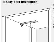
Can be post-installed to existing counters without processing. Simply by pressing against the supplied mounting template, installation position can be easily determined.
